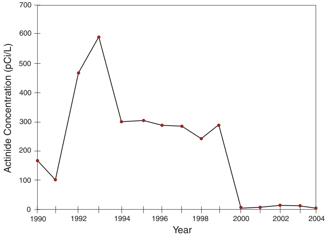
FIGURE 3.1a Actinide (Pu-238, Pu-239, Am-241) concentrations in effluent from the RLWTF. Releases of actinides have decreased significantly after upgrades to the facility in 1999. The concentration units of picocuries per liter (pCi/L) are 1000 times smaller than those in the figure for tritium below. These actinides have much longer radioactive half-lives than tritium, so they are usually of greater concern for groundwater protection.
